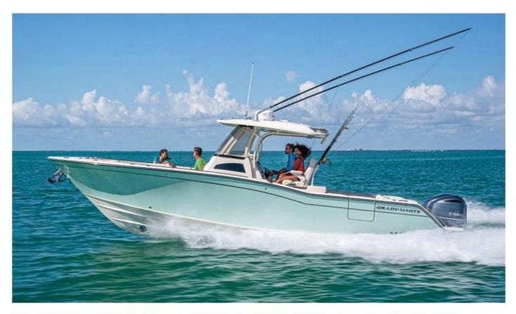
LOA: 31'2" | Beam: 10'9" | Fuel Capacity: 327 gal. | Dry Weight: 8,500 lb. plus power | Max HP: 700 |
