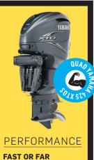
Running wide open, the 456 flirts with 60 mph. At 3,500 rpm, it cruises 345 miles at 30.7 mph.
