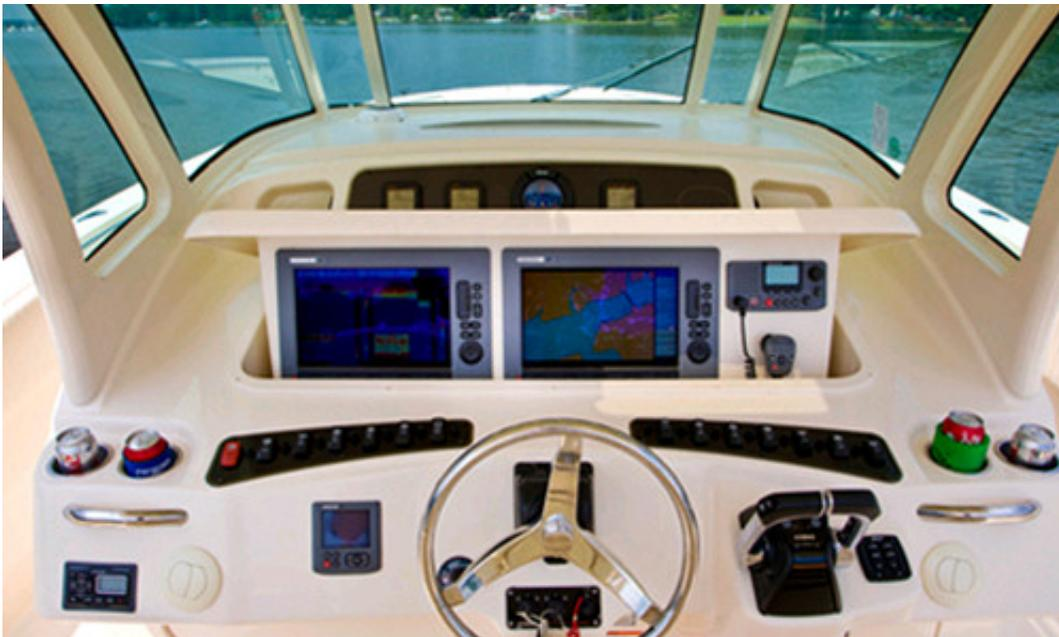
Electronics live in an enclosure that opens and closes electrically, with room for two big multifunction displays. There's an electronics box overhead, on the underside of the stylish T-top, standard equipment on the Canyon 366. Its frame is painted aluminum, and it's fitted with LED lights, stereo speakers and an overhead hatch.
