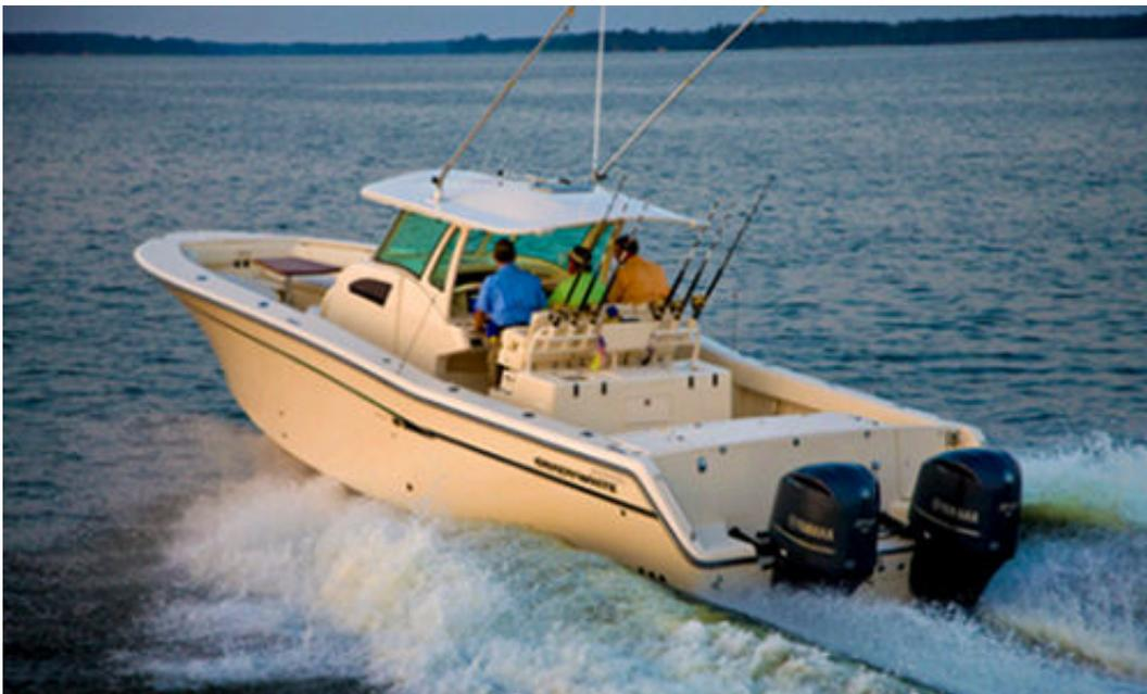
It's common to find triple outboards on a center-console this size, but sticking with twins might be best if top speed isn't your goal: Grady-White tests show almost identical optimum cruising speed and economy for twin- and triple-Yamaha 350 four-strokes. Both packages produce a shade over 30 mph (48.3 kph) optimum cruise, at about 1 mpg (.43 kpl).
