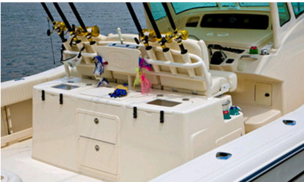
Grady-White calls their helm seating a "Deluxe Lean Bar." It includes a complete rigging station with a freshwater sink and 164-qt. (155.2 l) cooler, knife and pliers holders, lure holder and a 41-gallon (155.2 l) livewell. There are lockable tackle drawers and stowage lockers, and a 6-rig rocket launcher. All this is standard, but you can get...
