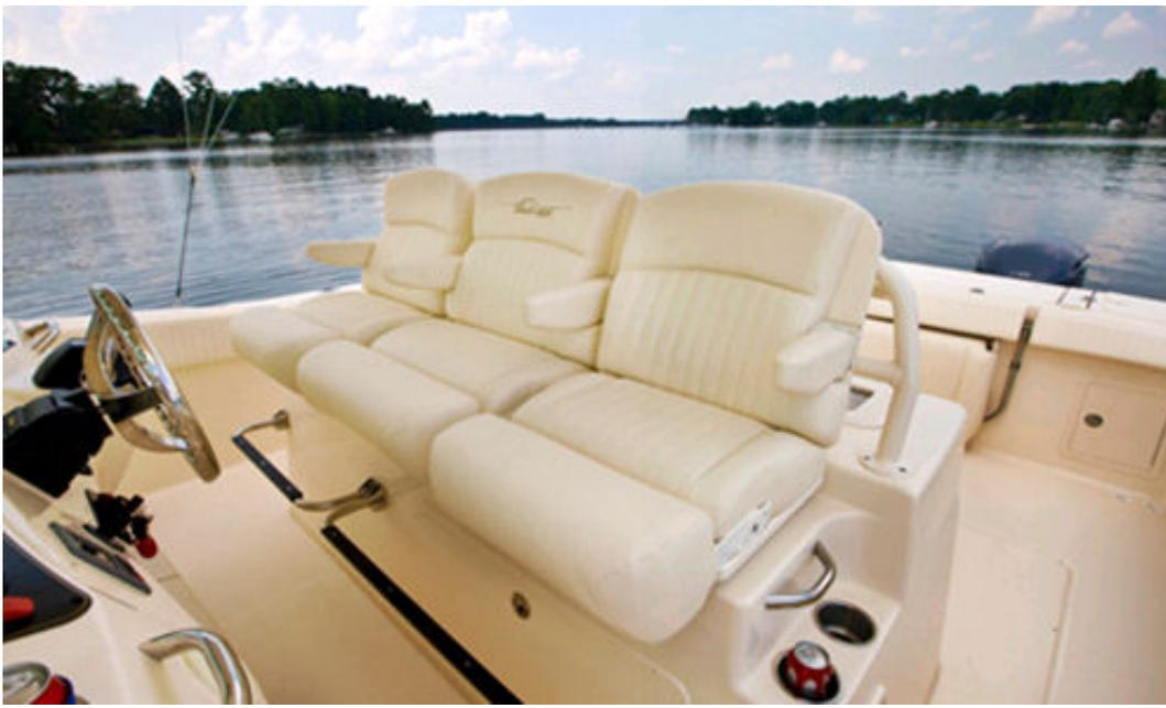
One advantage of a boat this size is plenty of beam, enough to fit triple seats at the helm and leave enough room to pass easily on either side when fighting a fish. We like the armrests to keep folks from sliding, the grabrails next to the seats and on the helm, and the full-width footrests.
