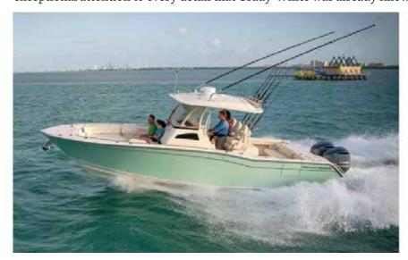
The Canyon 326 is a prime example. Built on Grady's proprietary SeaV2 hull—developed by the legendary C. Raymond Hunt design team—it blends the seakeeping attributes of a deep-vee with the fuel efficiency and performance of a modified-vee hull. Grady-White accomplished this by progressively varying the hull deadrise from 20 degrees at the transom to 30 amidships to an extremely sharp entry at the bow. The four strakes generate lift and a moderate chine knocks down spray.
