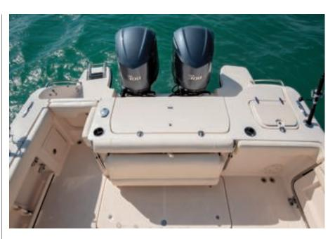
Above: The cockpit features tuna and boarding doors, a livewell, foldaway bench seating, and an 80-gallon fish box. Below: The standard hardtop comes with plenty of storage and is judiciously designed.
