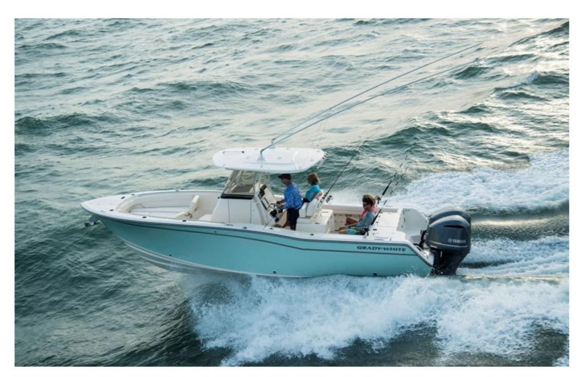
LOA: 26 ft. 10 in.; Beam: 9 ft. 6 in.; Draft: 23 in.; Deadrise: 20 deg.; Max Power: 600 hp Courtesy Grady-White Boats
