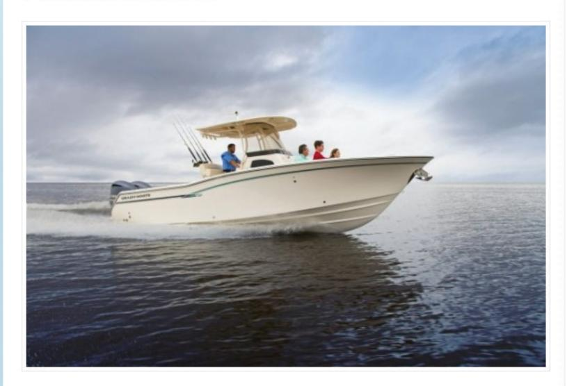
Grady-White's new Canyon 271 FS (forward-seating) offers comfort and versatility with port and starboard bow seating atop a pair of 85-quart insulated, overboard draining fishboxes. A casting platform insert option heightens the boat's fishability.
