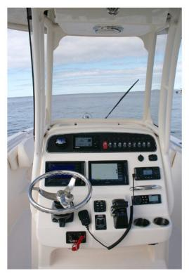
Under these, on the dash proper, are a brace of Garmin MFDs, a VHF, controls for the anchor and trim tabs, a USB charger and DC outlet, and the Fusion stereo. There is a stainless steel hand grip for the passenger and well padded seats and a footrest make it equally comfortable to sit as to stand.
