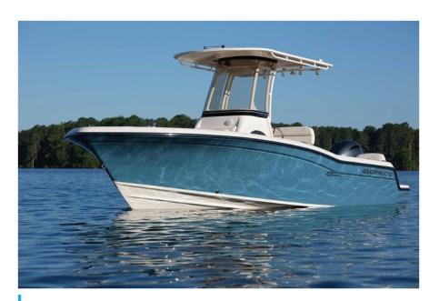
Beam Amidships: 8'6" (2.59 m) | Center Line Length (w/o Engine): 21'3" (6.48 m) (swim platforms not included) | LOA w/Swim Platforms: 23'6" (7.16 m) | Bridge Clearance: 6'7" (2 m), w/T-top: 7'7" (2.31 m) | Cockpit Depth: 25" (0.64 m) | Hull Draft: 16" | Transom Deadrise: 19 degrees (SeaV2® progression) | Maximum HP: 250 (187 kW) | Fuel Capacity - Standard: 80 gal. (303 l)
