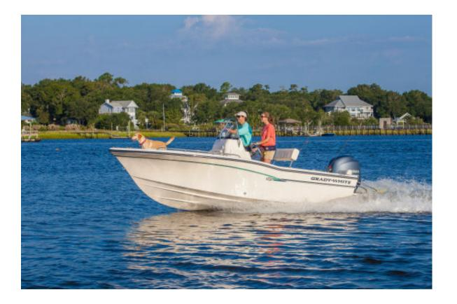
The Grady-White Fisherman 180 has a length of 17'10" (5.44 m), a beam of 7'5" (2.26 m) and a displacement of 2,150 lbs. (975 kg).
