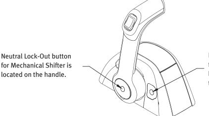
Neutral Lock-Out button for Electronic Shifter is located on the aft side of the unit. If your boat is equipped with Helm Master<sup>™</sup> there is a feature that is similar to a neutral lockout on other boats. When activated, the free throttle button allows opening the throttles on all engines without engaging the forward or reverse gear. The active indicator will be illuminated during operation. See Yamaha Helm Master<sup>™</sup> Operation Manual for detailed instructions.
