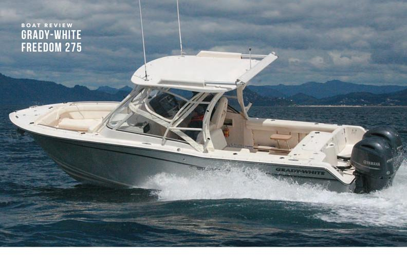
The twin Yamaha 200s were amazingly responsive, especially in the mid-range. Powered by twin Yamaha F200 four-strokes, this solid GRP 8.5-metre vessel can carry almost 700 litres of fuel and boasts a trailerable weight of 3100kgs.
