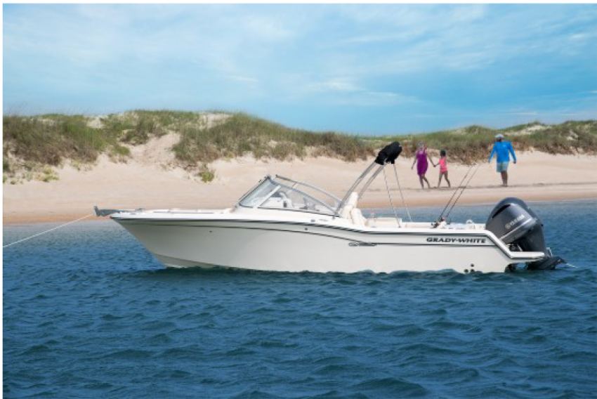
Grady-White's all new Freedom 235 has an LOA of 23'7" (7.18 m) and a beam of 8'6" (2.59 m).
