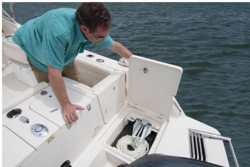
The starboard swim platform storage, housing a stern anchor, with matching storage to port. Never anchor from the stern offshore.
