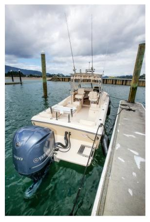
Not that this is a hard boat to keep clean, with both raw water and freshwater (38-litre tank) washdown facilities in the cockpit and selfdraining decks. A freshwater shower/washdown in the cockpit is not just great for divers, but also for rinsing salt off fishing tackle at the end of the day.
