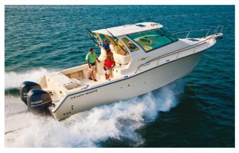
SPECS: LOA: 36 ft. 7 in. • Beam: 13 ft. 2 in. • Transom Deadrise: 20 deg. • Draft: 29 in. Dry Weight: 14,919 lb. • Max Power: 1,050 hp
