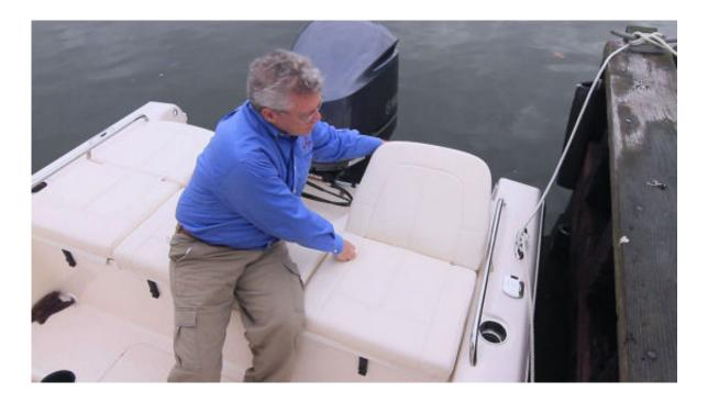
Lifting the seat back from the aft position, rather than having it fold down onto the seat itself, deploys these jump seats. This allows the space underneath to be more fully utilized.
