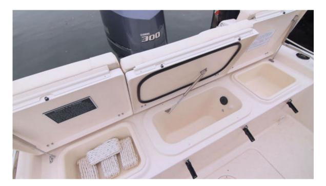
The transom seats lift to reveal storage bins port and starboard and an insulated, self-draining 51 quart (48.3 L) compartment that can be used as a fishbox, beverage cooler, or for more storage.
