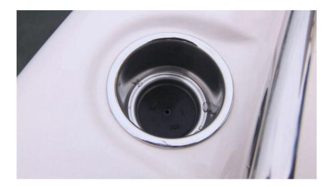
See the drain hole at the bottom of this drink holder? A hose connects to it to allow condensation to run into the cockpit.
