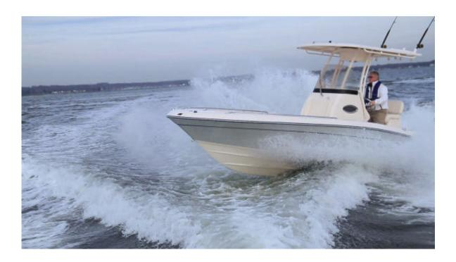
The 251 CE's sharp entry cuts through waves rather than bouncing over them. Here we can see how the spray is thrown wide and low contributing to the dry ride.
