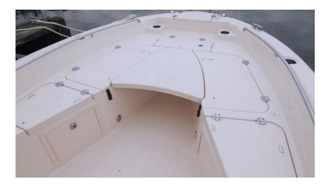
At the bow there are two 74-quart fishboxes, port and starboard. Just behind are the lifting seat backs which create chaise seating.
