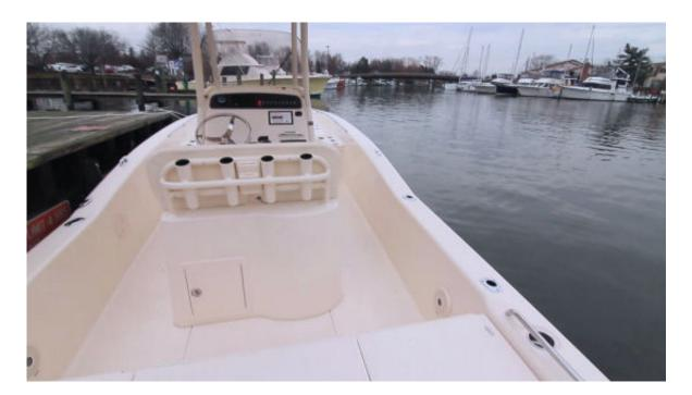
Rod holders are in the caprails, at the bow, behind the leaning post, and at the rear of the T-top.
