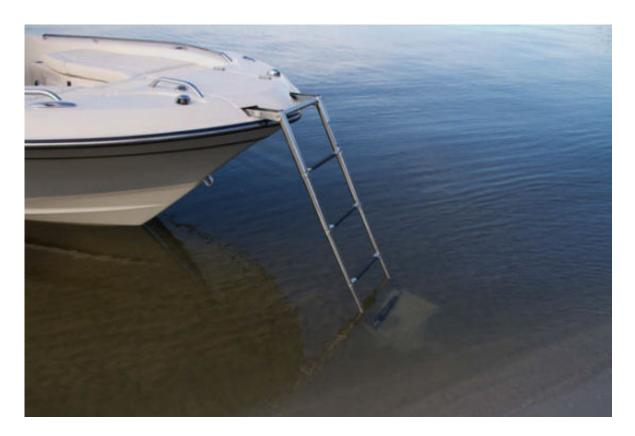
Standard equipment on the Grady-White 251 CE is a 4-step beach boarding ladder on the bow. This gives the boat lots of added utility and combines with the boat's 14" (.36 m) draft makes getting off and on easy, and even dry in the right locations.
