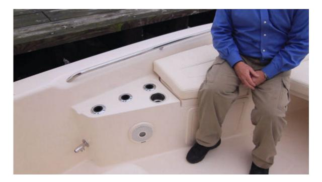
There's no shortage of stainless steel on the 251 CE, and that includes the raw water washdown spigot at the bow. The three vertical rod holders (and the three on the starboard side) are standard.
