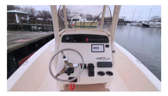
Grady-White created a good looking helm for the 251 CE and we also appreciated the ergonomics. Note that the supports for the optional T-top are affixed to the side of the console and not mounted to the deck where they will stub toes and take up space.
