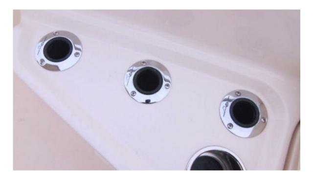
All the rod holders are flush mounted and stainless steel.
