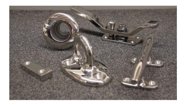
The stainless steel is all 316-grade alloy which maintains a high level of nickel to better resist staining. It's double polished and double passivated making it unreactive by coating the surface with a thin inert layer. This is how the shine is maintained for a longer period.
