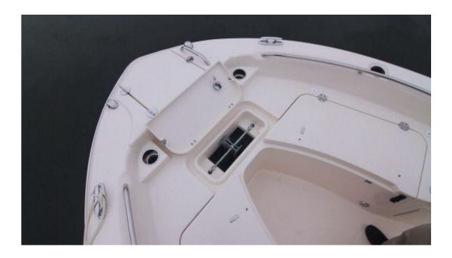
Fully forward is a dedicated locker for a Danforth-type anchor. Note the port and starboard running lights which are separate and larger than what we normally see on this type of boat.
