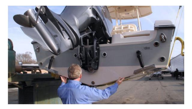
The 16-degree deadrise at the transom and her wide chine flats make the 251 CE fast out of the hole, fuel efficient at best cruise and fast at the top end. In addition, these two attributes dampen roll, making the 251 CE more comfortable than deep-V designs.
