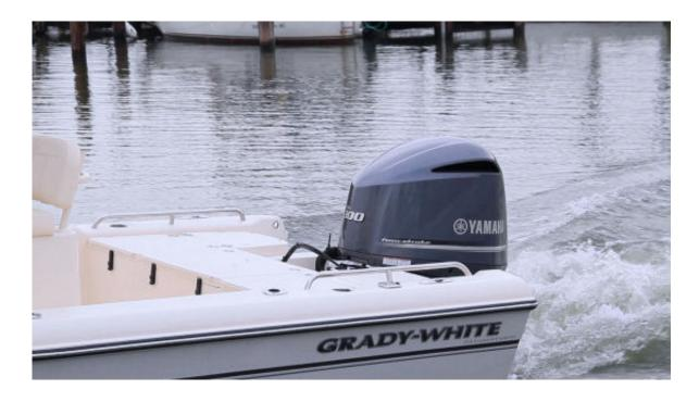
Our test boat was powered with a Yamaha F300 outboard.
