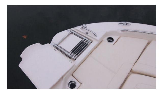
The 251 CE is designed for heading to remote beaches. Here's a bow reboarding ladder for when we tuck the bow against the shore. There's even a stainless grab handle alongside. This is the only center console that we have ever seen with a bow boarding ladder.
