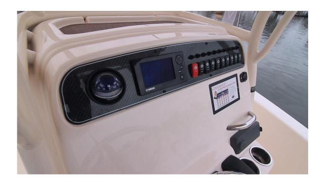
In the center of the panel is the Yamaha engine display allowing selectable information. There is plenty of real estate for one, large multi-screen display, or for two smaller screens.
