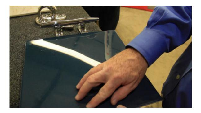
The 251 CE comes with a choice of 6 different hull colors. The dark colored Grady White hulls are painted rather than coloring the gel, which is how the builder handles lighter colors. This dual approach permits a more controlled and a glossier shine.
