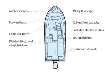
Beam Amidships: 8' (2.44 m) Bridge Clearance: 6'2" (1.88 m) w/Hardtop: 8'4" (2.54 m) Center Line Length: 22'2" (6.76 m) Hull Draft: 16" (0.41 m) Maximum HP: 300 (224 kW) Weight w/o Engine: 226 (standard transom): 3385 lb. (1535 kg) 228 (Grady Drive transom): 3510 lb. (1592 kg)
