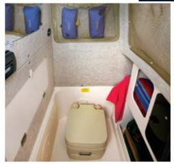
Lockable stand up console head enclosure with storage shelves and hanging locker; shown with optional portable head
