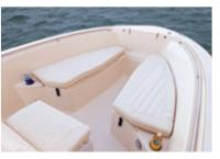
101-qt. (96 l) port and starboard forward insulated fish boxes with ob drain. Access to bow at deck level. Console forward seating with removable 72-qt. (68 l) cooler.
