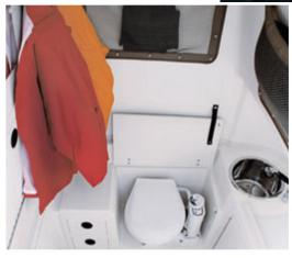
Lockable console with sink, storage and fold down cover over marine head with macerator, 10-gallon (37.9 l) holding tank and pump out
