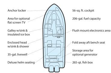
Beam Amidships: 9'11" (3.02 m) Bridge Clearance w/Hardtop: 9'9" (2.97 m) Center Line Length: 28'6" (8.69 m) Length Overall (w/pulpit): 29'9" (9.07 m) Hull Draft: 24" (0.6 m) Maximum HP: 600 hp (448 kW) Weight w/o Engines: 7650 lb. (3470 kg)
