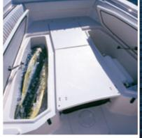
Bow insulated fish boxes with removable optional casting platform insert
