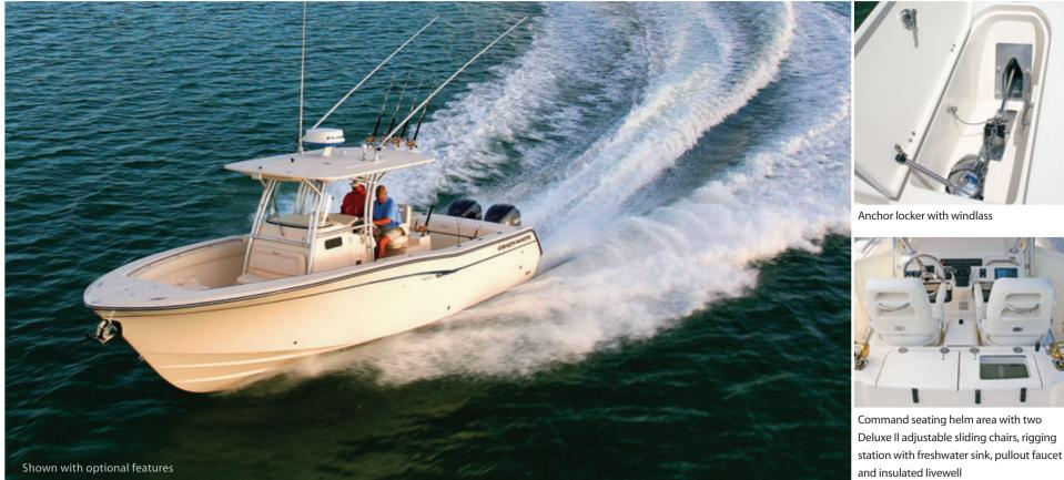
Beam Amidships: 10'7" (3.23 m) Bridge Clearance: 7'3" (2.21 m) w/T-top: 9'4" (2.84 m) Center Line Length: 30'6" (9.30 m) Hull Draft: 21" (0.53 m) Maximum HP: 700 (522 kW) Weight w/o Engines: 6950 lb. (3152 kg) Anchor locker 150-qt. port and starboard fish boxes Lockable console with stand up head area, shower, sink and storage areas Electromechanically operated electronics enclosure
