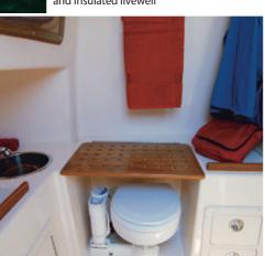
Lockable console with sink, storage and fold down cover over marine head with macerator, 10-gallon (37.9 l) holding tank and pump out
