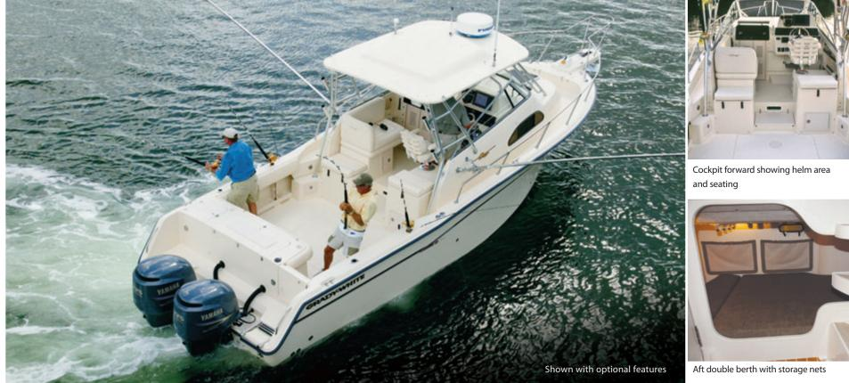
Beam Amidships: 10'7" (3.23 m) Bridge Clearance w/Hardtop: 9'9" (2.97 m) Center Line Length: 30'6" (9.30 m) Length Overall (w/pulpit): 32'7" (9.93 m) Hull Draft: 23" (0.58 m) Maximum HP: 700 (522 kW) Weight w/o Engines: 8221 lb. (3729 kg)
