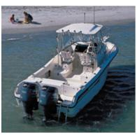
Cockpit forward showing transom door and integrated swim platform with ladder
