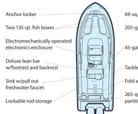
69-sq. ft. cockpit 205-gal. fuel capacity 45-gal. livewell Tackle locker w/trays Fold away aft bench seat 265-qt. fish box w/removable partition and ob drain
