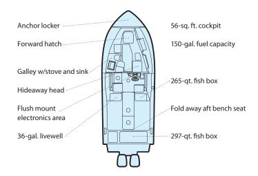
Beam Amidships: 9'3" (2.82 m) Bridge Clearance: 6'5" (1.96 m) w/Hardtop: 8'8" (2.64 m) Center Line Length: 23'5" (7.14 m) Hull Draft: 20" (0.51 m) Maximum HP: 400 (298 kW) Weight w/o Engine: 232S: 4538 lb. (2058 kg) 232D: 4605 lb. (2089 kg)
