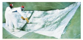
Skilled craftsmen apply hand laid fiberglass with precisely the right thickness and resin ratios. Top quality components assembled with skill result in quality, reliability and performance over the long haul.
