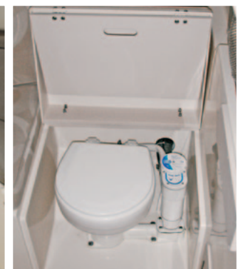
Head area in lockable cabin, with fold down cover; optional electric marine head shown
