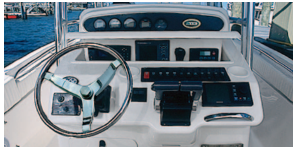
Helm console with electromechanically operated lockable electronics enclosure
