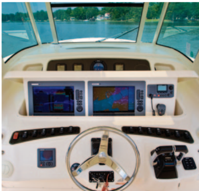
Electromechanically operated electronics enclosure (enclosure up)
