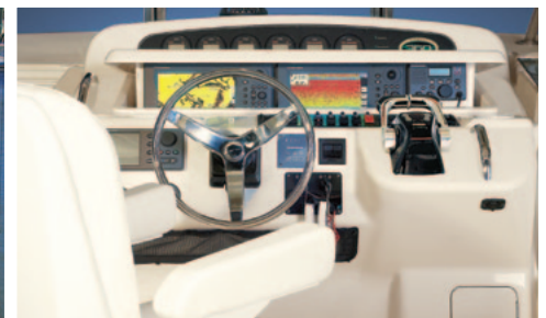
Helm includes deluxe adjustable seating, power assisted tilt steering, electronically programmable throttles with engine synch mode, electromechanically operated electronics enclosure, and easy-access accessory fuse compartment.
