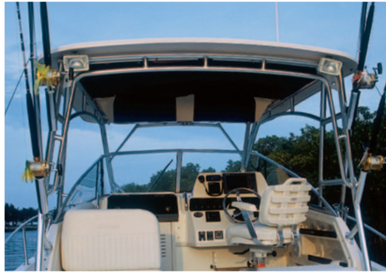
▲ Cabin model hardtop with lockable radio box(es), spreader light(s), side rod holders and overhead storage net (optional models 22'-25', standard 29'-36')
