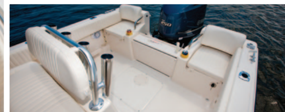
Optional deluxe lean bar with rod holders; aft cushioned seats and fold down motorwell bulkhead; optional cockpit bolsters
