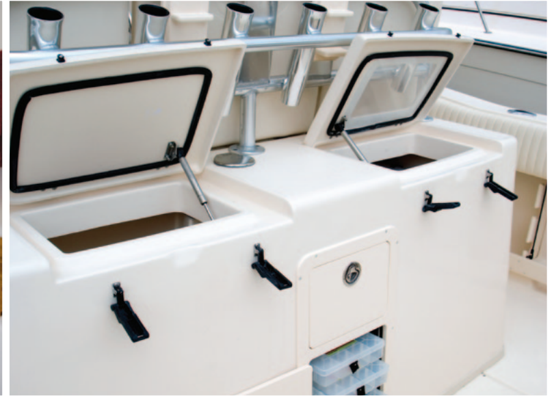
Rigging station with freshwater washdown, 104-quart cooler, tackle drawers, storage, rod holders and knife & pliers holder
