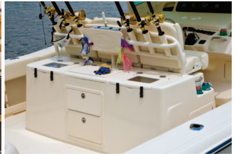
Lean bar with 41-gal. (155.2 l) insulated raw water livewell with see-through lid, light, full column distribution inlet and overboard drain (110 GPH pump) (4164 LPH); lure holder and rigging station with freshwater sink, shown with optional second livewell; available standard with 164-qt. (155.2 l) cooler
