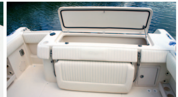
304-quart aft insulated fish box, transom door and folding aft bench seat
