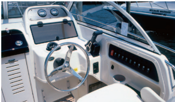
Helm station with lockable electronics box
