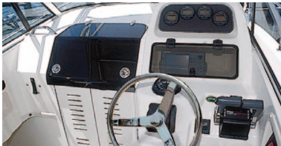
Helm station with lockable electronics box
