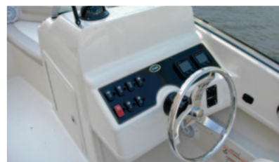
Helm station with flush mount electronics area
