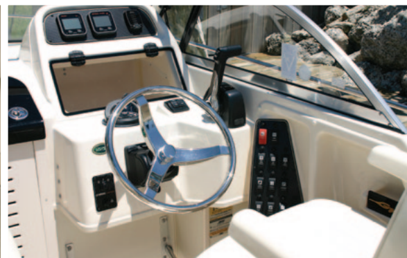
Helm station with lockable electronics box
