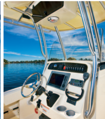
Helm showing footrest, flush mount electronics kit, acrylic windshield and optional T-top with radio box
