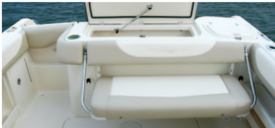
Aft fold away bench seating, 185-quart insulated fish box, and 128-quart cooler (32-gallon livewell optional)
