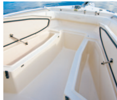
101-qt. (96 l) port and starboard forward insulated fish boxes w/ob drain. Access to bow at deck level.
