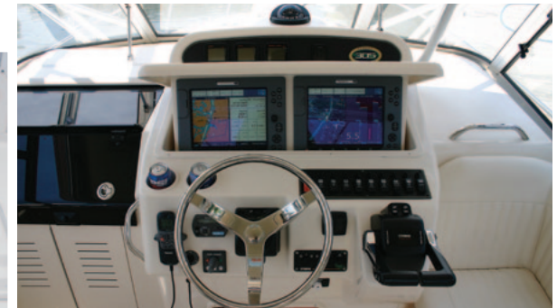
Helm station with electromechanically operated lockable electronics enclosure
