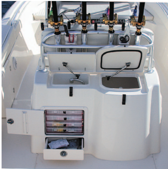
Lockable head enclosure with fold down cover, sink and storage
