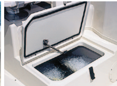
158-quart starboard insulated fish box with overboard drain
