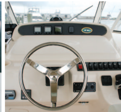
Helm console with electromechanically operated lockable electronics enclosure
