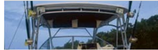
▲ Hardtop with lockable radio boxes, spreader lights, side rod holders and overhead storage net (optional for cabin models 22'-27', standard for 28'-36')
