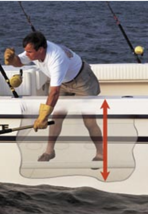
Step aboard a Grady and notice the high gunwales. These provide safety when you lean out over the water and are a real assurance when seas are rough.
