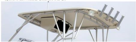
▲ Hardtop with lockable radio box, spreader lights and rod holders (208)
