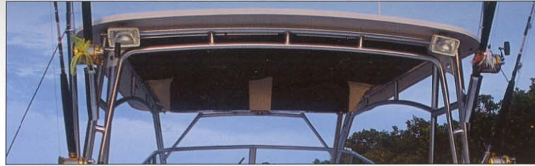
▲ Hardtop with lockable radio boxes, spreader lights, side rod holders and overhead storage net (for models 22' and up)
