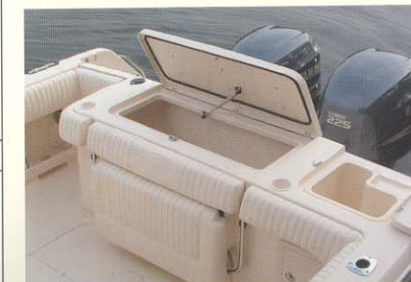
Fold away bench seat, transom door, fish box and lift out box
