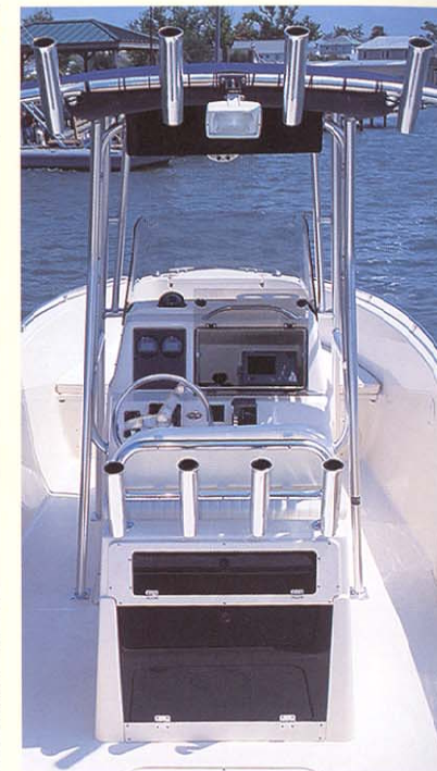
Cockpit forward with optional T-top and lean bar with tackle and bulk storage
