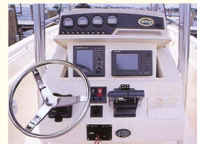
Console with electro-mechanically operated electronics enclosure
