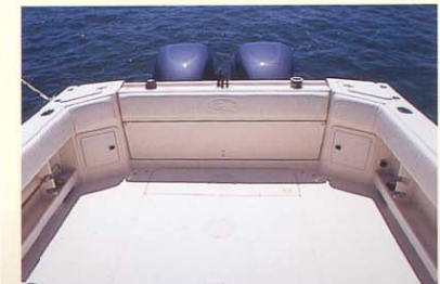
Aft cockpit with fold down motorwell bulkhead, aft deck lift out boxes and horizontal rod storage
