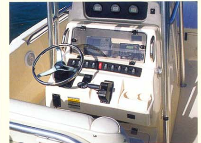
Console with lockable electronics box
