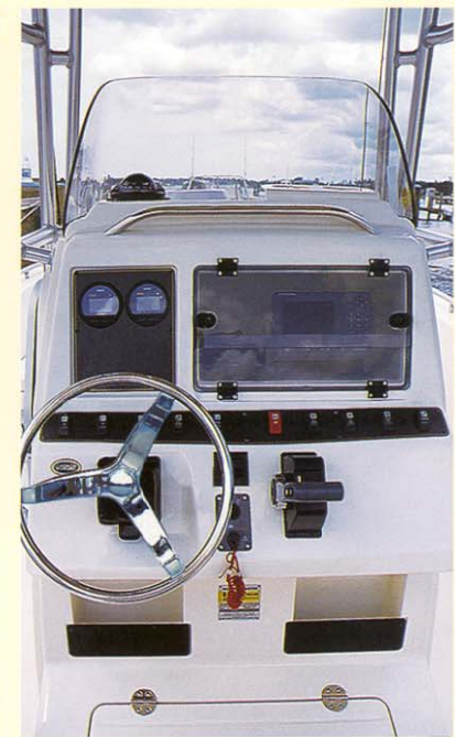
Console with lockable electronics box, footrest and storage compartment
