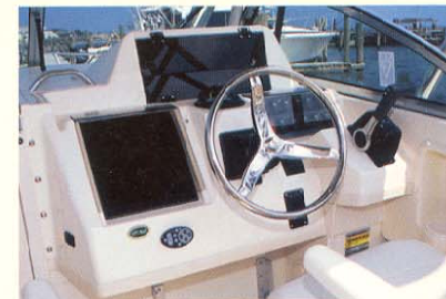
Helm station with lockable electronics box
