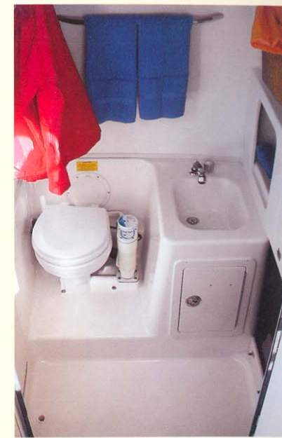
Lockable head enclosure with sink, shower and storage
