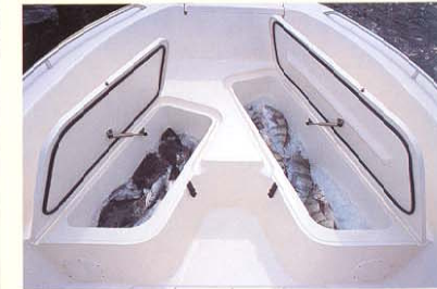
Insulated bow fish boxes with overboard drains
