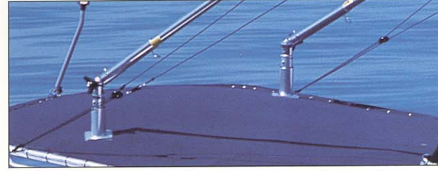
▲ Outrigger kit, Radial Top Gun T-top Mounted
