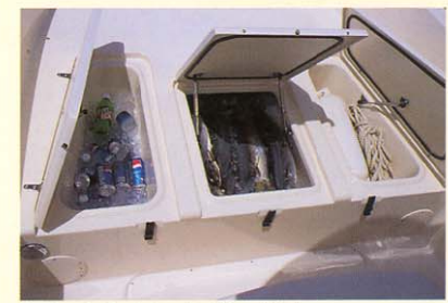
Casting platform's insulated bow fish boxes with overboard drains
