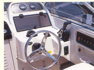
Helm station with lockable electronics box
