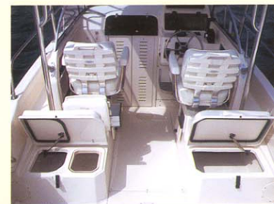
Cockpit forward with divided port insulated fish box
