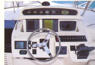
Helm station with electro-mechanically operated electronics enclosure
