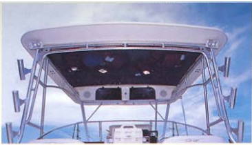
Hardtop with net storage, electronics enclosure and rod holders
