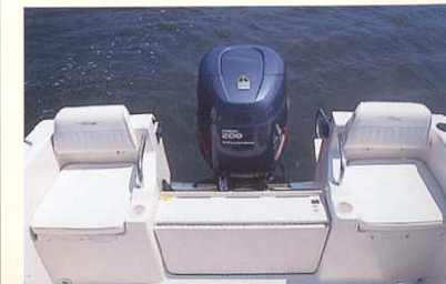
Aft cockpit with fold down motorwell bulkhead
