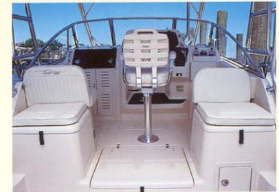
Helm area with removable seat backs and vertically and horizontally adjustable helm chair
