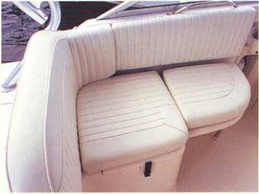
Port helm seating area features a folding seat and insulated ice box
