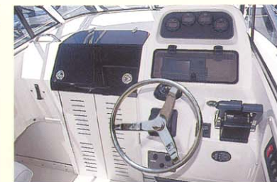
Helm station with lockable electronics box
