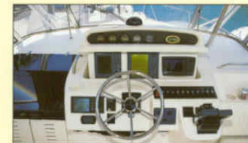
Helm station w/electro-mechanically operated electronics enclosure
