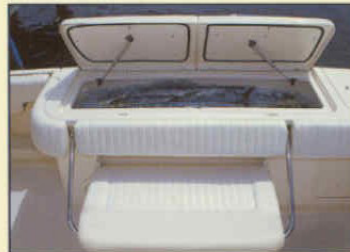
270-qt. aft deck insulated fish box; fold away aft bench seat w/cushion
