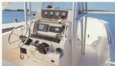
Center console with lockable electronics box
