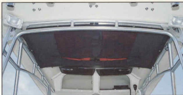
▲ Hardtop with lockable radio box, spreader lights and overhead net storage
