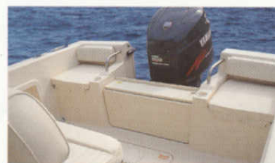
Aft cockpit with fold down motorwell bulkhead
