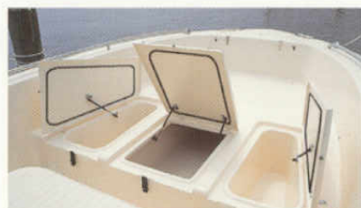
Casting platform with insulated fish boxes
