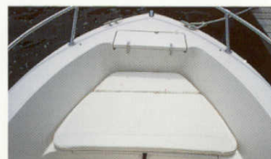
Bow casting platform w/optional forward platform cushion
