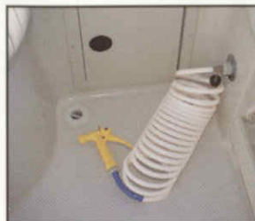
▲ Saltwater washdown w/ Hydra-Koill hose
