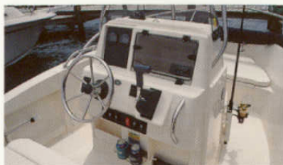
Console with lockable storage and electronics box
