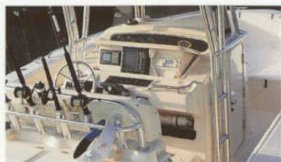
Console with electro-mechanically operated electronics enclosure and rigging station
