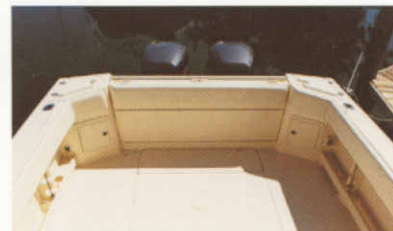
Aft cockpit with fold-down motorwell bulkhead
