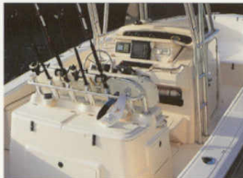
Console w/electro-mechanically operated electronics enclosure & rigging station
