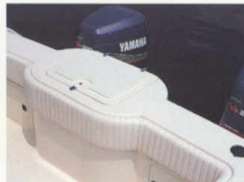
Aft cockpit w/42-gal. raw water livewell
