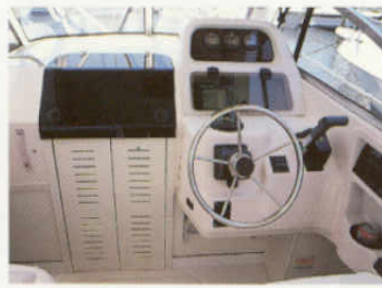
Helm station w/lockable electronics box
