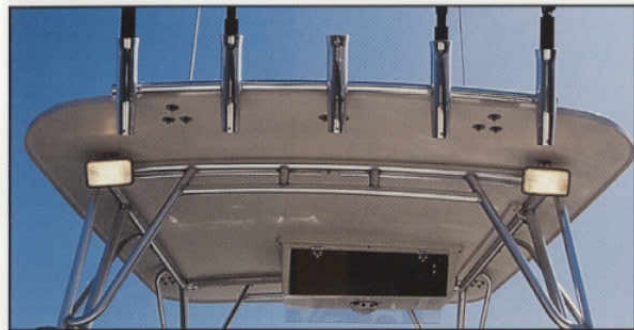
▲ Hardtop with lockable radio box, spreader lights and rod holders
