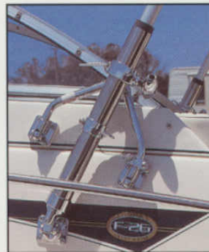
▲ Outrigger kit, cabin side mounted
