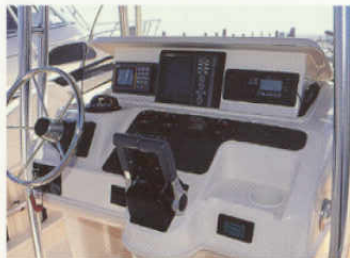
Console w/electro-mechanically operated electronics enclosure (shown in up position)
