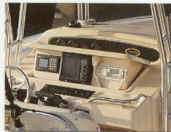
Console w/electro-mechanically operated electronics enclosure (up)
