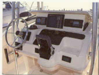
Console with electro-mechanically operated electronics enclosure (up)
