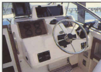
Helm station w/lockable electronics box
