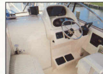
Helm station w/sliding cabin door
