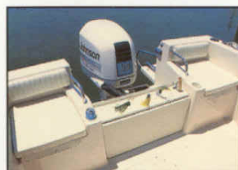
Fold down motorwell bulkhead
