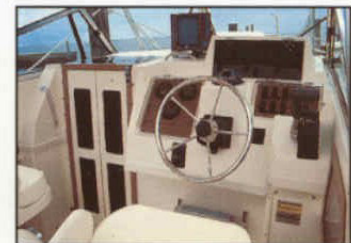
Helm station w/lockable electronics box
