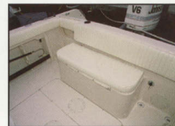
Aft bench seat with transom door
