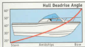
The continuously variable vee cuts through waves while the flatter stern provides stability.
