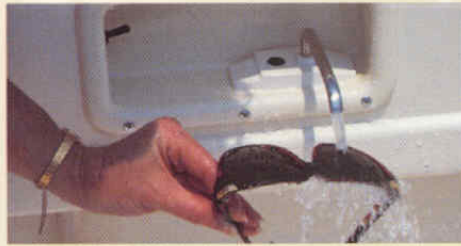
▲ Gunwale mounted freshwater system
