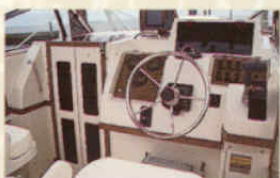
Helm station with lockable electronics box
