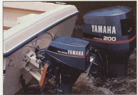
▲ 9.9 hp auxiliary kicker engine
