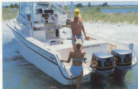
Integrated outboard mounting system
