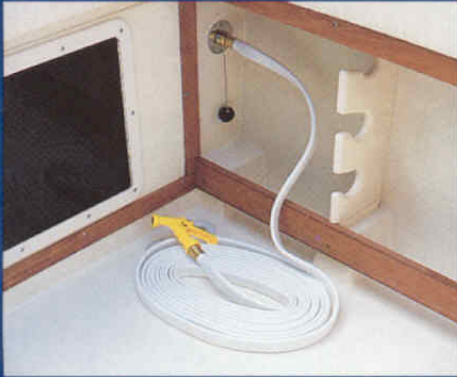
Washdown system with hose
