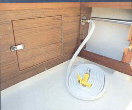
Washdown system with hose
