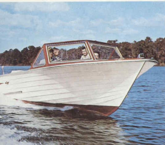
Wide beams and flared bows made lapstrake hulled wooden Grady-Whites favorites with fishermen.
