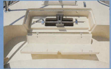
Bow anchor locker
