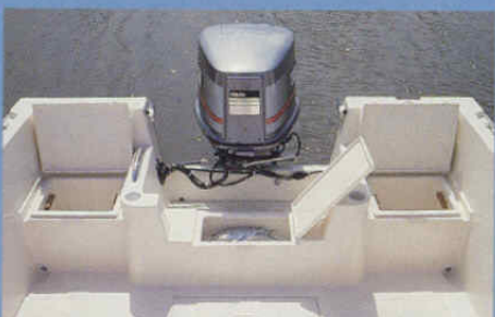
Aft wells (204-C)
