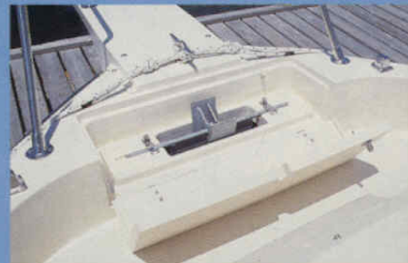
Bow anchor locker
