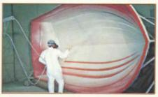
The finest NPG gelcoat is applied in our dust-free spray booths giving a smooth, durable finish to the hull and deck.
