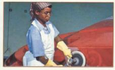
The mold determines the boat's shape and finish, so we carefully inspect each one, then polish it to insure a smooth finish.
