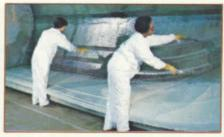
3. Hand-laid fiberglass mat and woven roving means a stronger, safer hull and deck. The hand lay-up process gives control of the fiberglass-toresin ratio, insuring the uniform strength we require.
