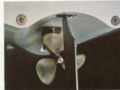
Jim Wynne-designed propeller pocket (256)
