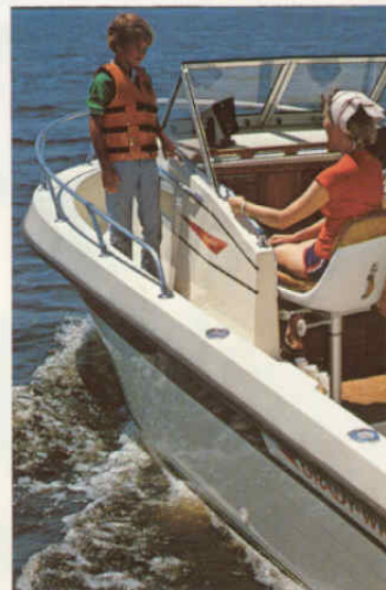
Recessed non-skid walkway
