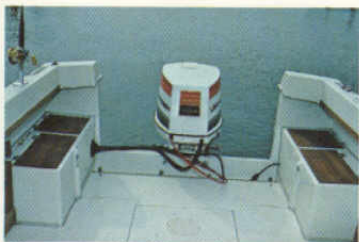
Aft motor well bulkhead, down
