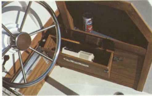
Lockable radio box at helm station
