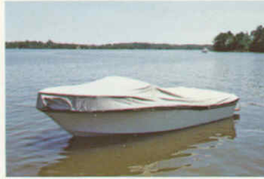
Mooring cover (canvas): Covers and protects entire deck and interior of boat.
