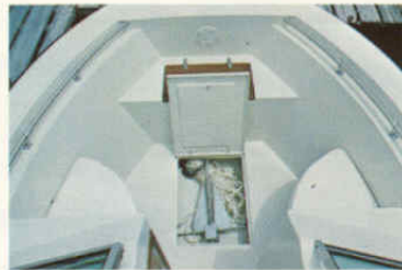
Bow anchor locker
