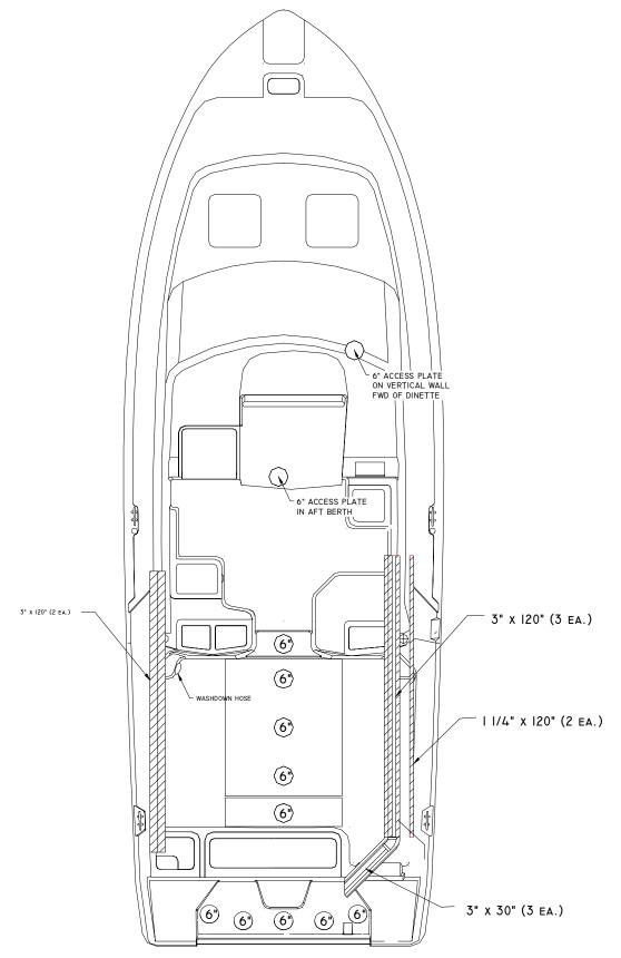
**ACCESS PLATE AND RIGGING TUBE LOCATIONS**
