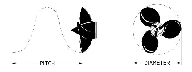
Pitch = 17Diameter = 14Pitch and Diameter are the two basic dimensions of a propeller.<br/>Example of propeller dimension: 14 x 17
