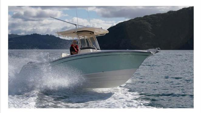
They design deep vee, solid GRP hulls with high freeboard. They use only marine grade stainless steel for their fittings, put only the latest four-stroke Yamaha outboards on their transoms and ensure there are enough rod holders, live bait wells, ice boxes and drink receptacles for even the most successful and thirst-inducing of fishing expeditions.
