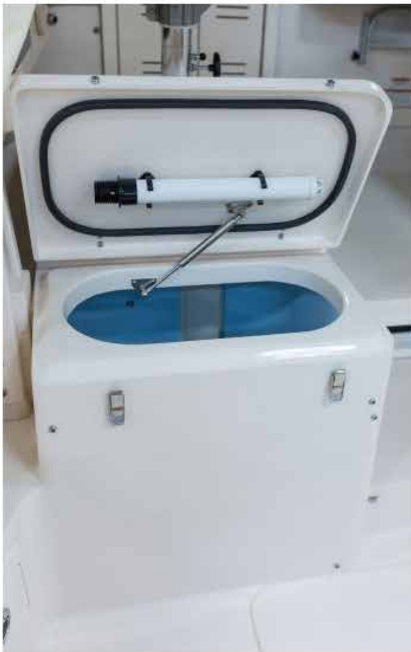
The cockpit livewell, which sits to port, just abaft the companion seat.
