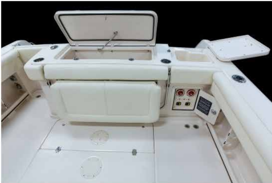
A view of the aft fishbox, removable storage tub on the port side for easy battery access and battery switches. We like the handy battery switches.
