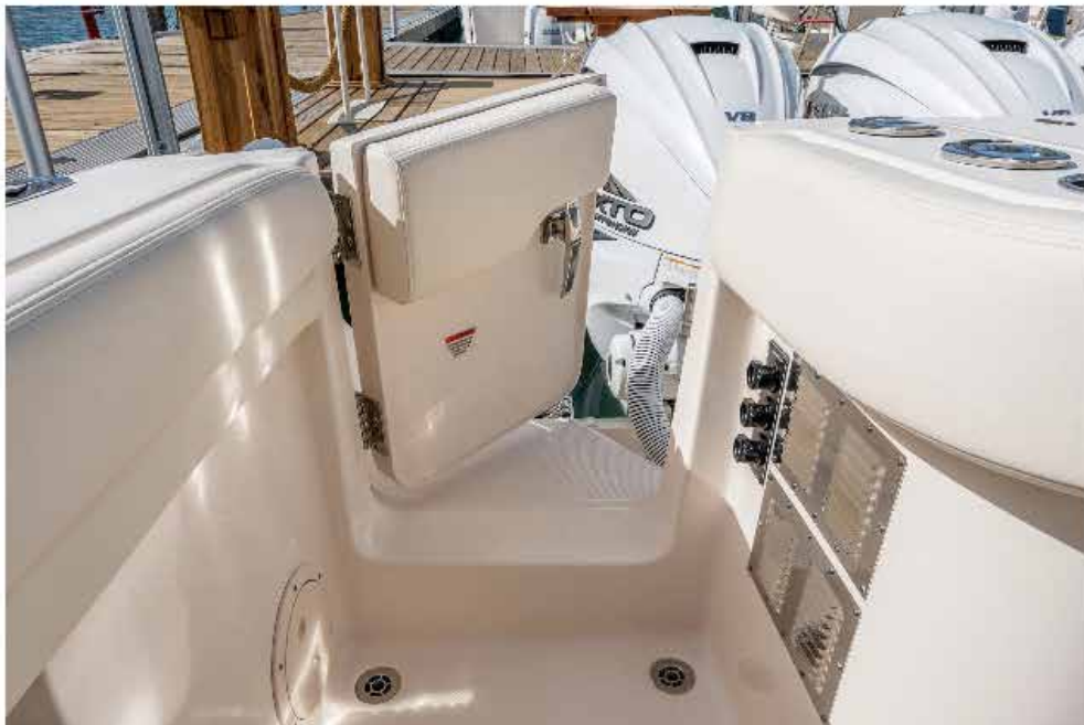
Typical of the hardware we saw throughout the Canyon 376, the transom door closes with a heavy-duty latch.
