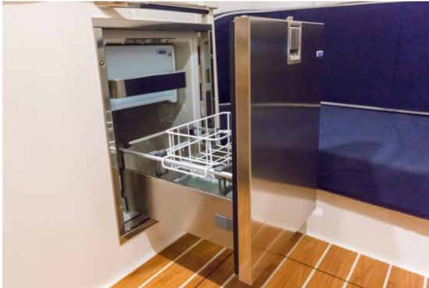
A drawer-style refrigerator that stays closed with a secure latch is a good idea for an offshore boat.
