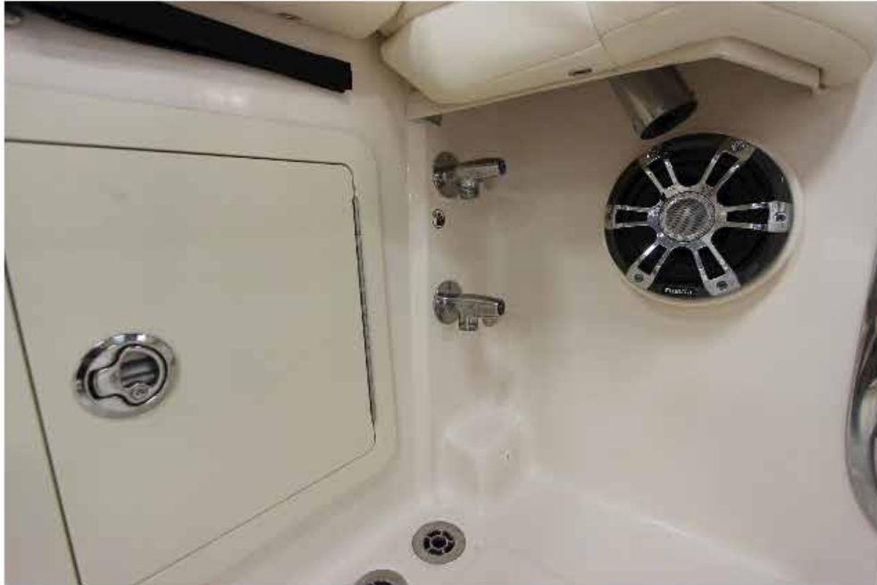
The fresh and raw water washdowns aft to port will facilitate cleaning the decks after a day of fishing.
