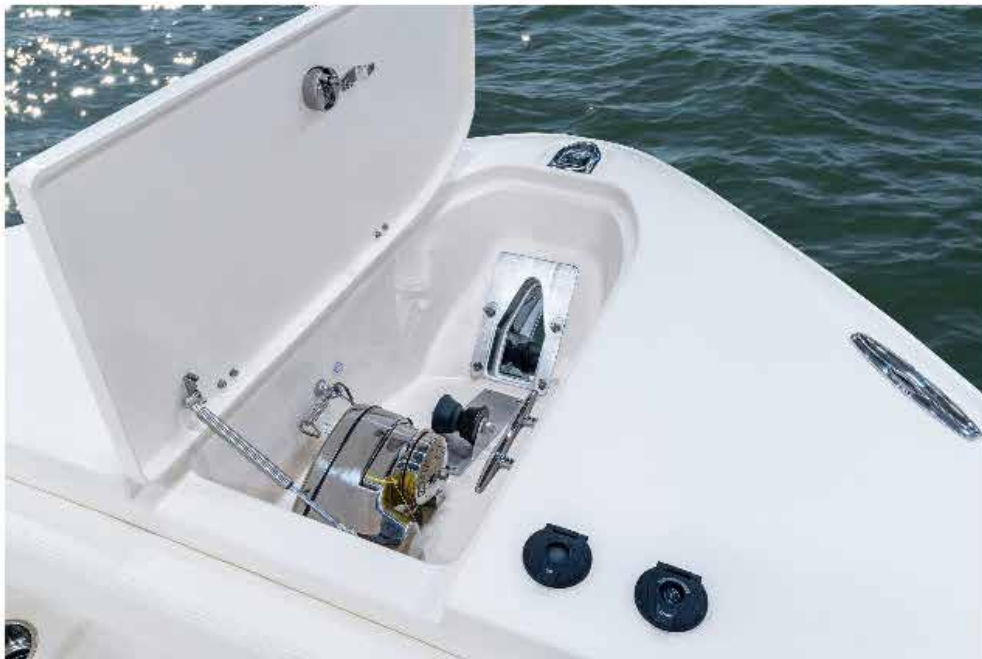
A windlass and a stainless-steel anchor chute come standard on the Canyon 376.
