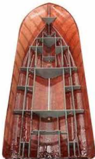
The Canyon 376 is built with composite coring for the stringers, bulkheads, and transverse braces, and the transom gets additional strength from these aluminum supports.
