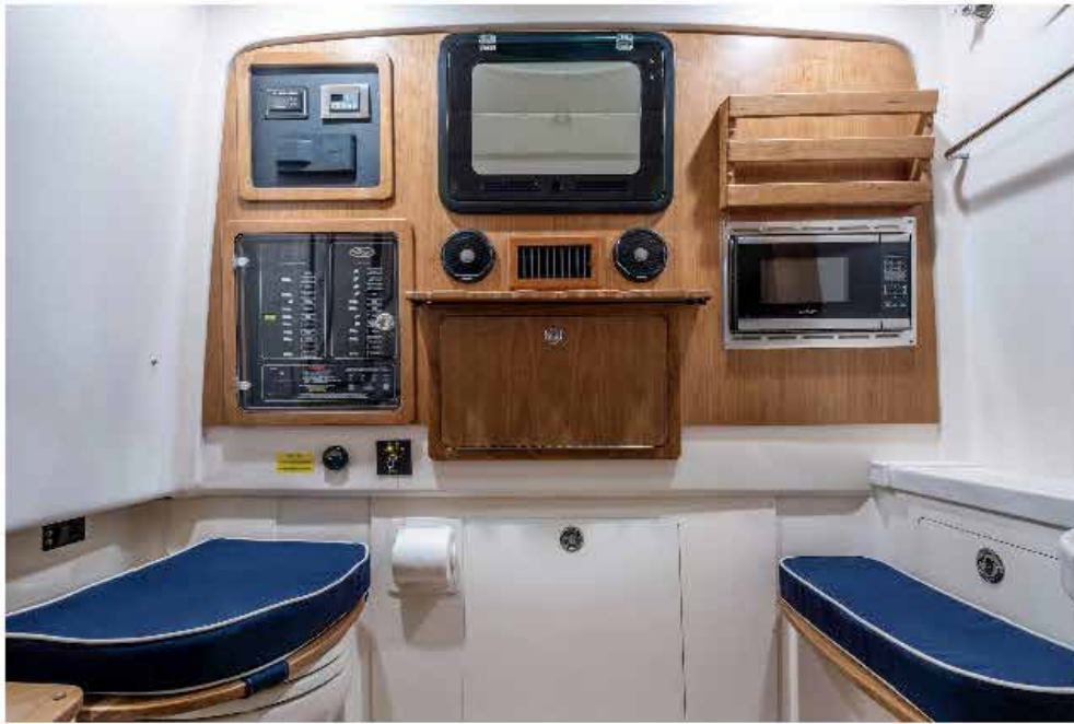
The upper panel in the cabin controls the stereo, the air conditioning, and the temperature for the optional refrigerated/freezer aft fish box.
