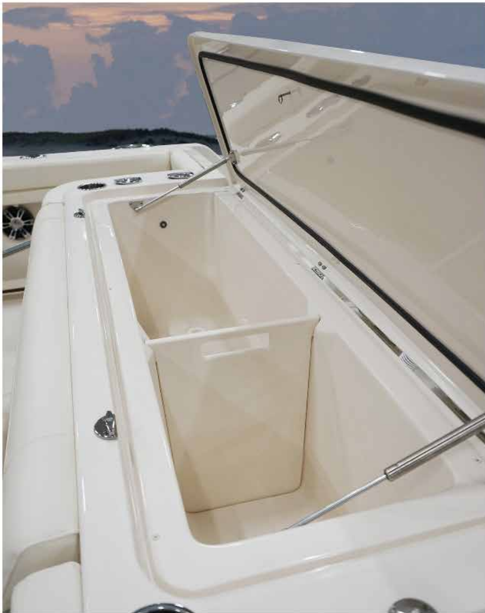
The hatch for the aft fish box opens on twin stainless steel pneumatic struts and closes on a thick rubber gasket. It's capacity is 291 qts., it's insulated and self-draining.
