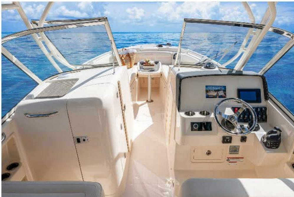
**Notice the windshield that has been made higher and wider for improved visibility. This model has the Helm Master joystick next to the wheel.**
