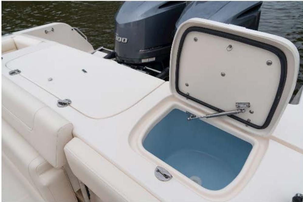
**The 32-gallon (121.13 L) livewell is colored blue and includes rounded edges to reduce the shock on live bait.**
