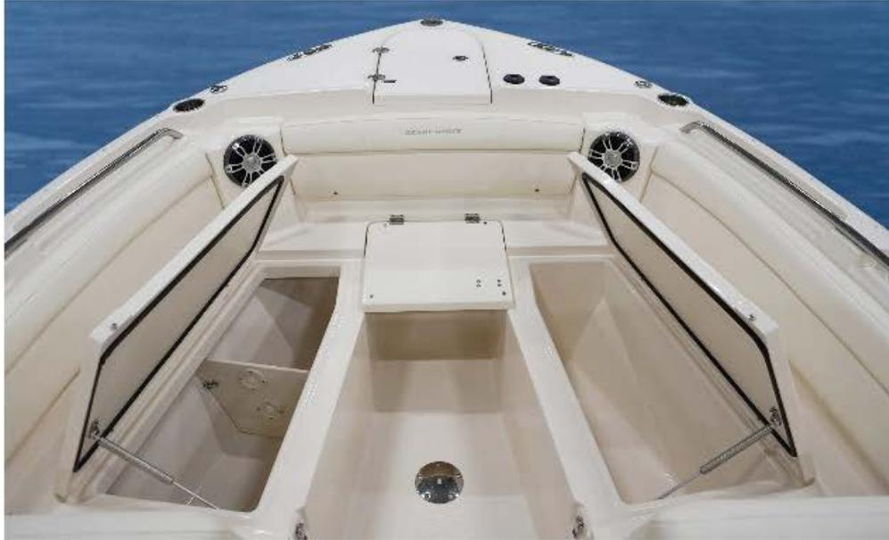
**Storage is under both bow seats. To port rod storage extends into the head compartment just behind. To starboard, an insulated box holds ice or fish.**
