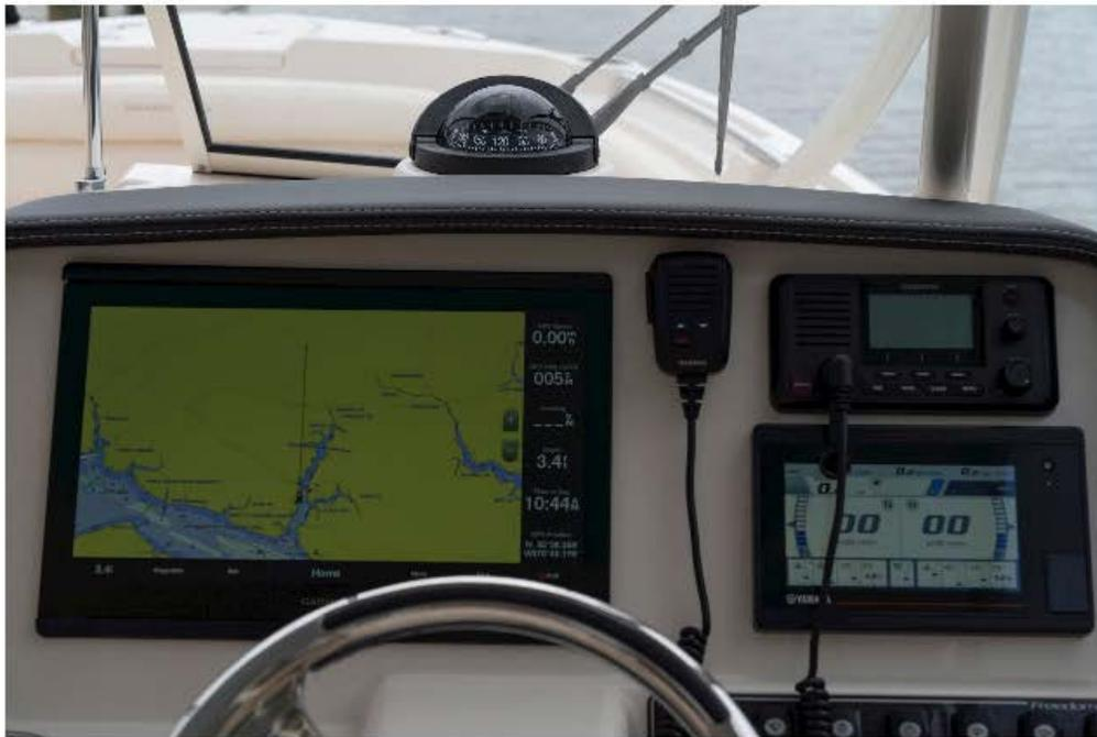
**With a larger helm console, the panel can now accommodate larger displays. This is a 17" (43.18 cm) Garmin sharing space with the Yamaha engine monitor and a Garmin VHF.**
