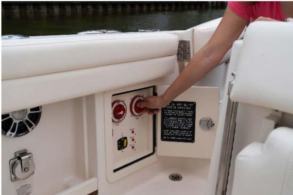
**Battery switches are right inside the cockpit entrance. Notice the shore power plug. It's part of an optional convenience package.**
