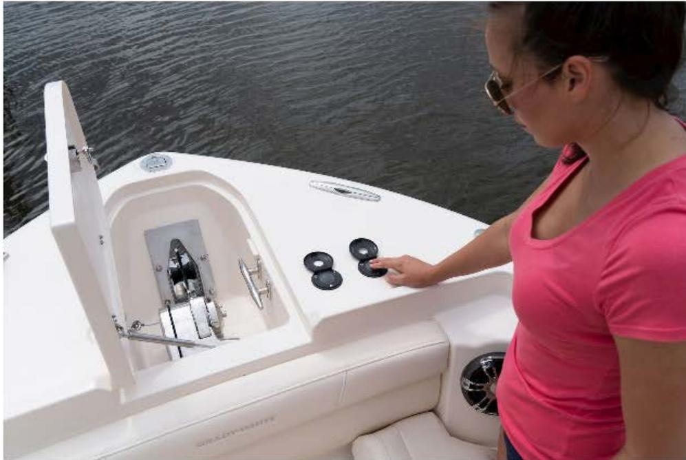
**The windlass is standard. Controls are to the side. Notice how the hatch is finished on both sides.**
