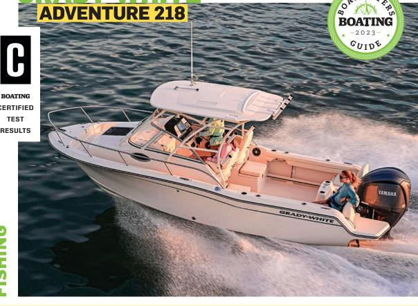
SPECS: LOA: 21'3" (23'3" with platforms) BEAM: 8'6" DRAFT: 1'4" (motor up) DRY WEIGHT: 3,650 lb. (no engine) PASSENGER/WEIGHT CAPACITY: 8/NA FUEL CAPACITY: 100 gal. HOW WE TESTED: ENGINE: Yamaha F250 XSB DRIVE/PROP: Outboard/SWS II 15.75" x 15" 3-blade stainless steel GEAR RATIO: 1.75:1 FUEL LOAD: 50 gal. CREW WEIGHT: 400 lb
