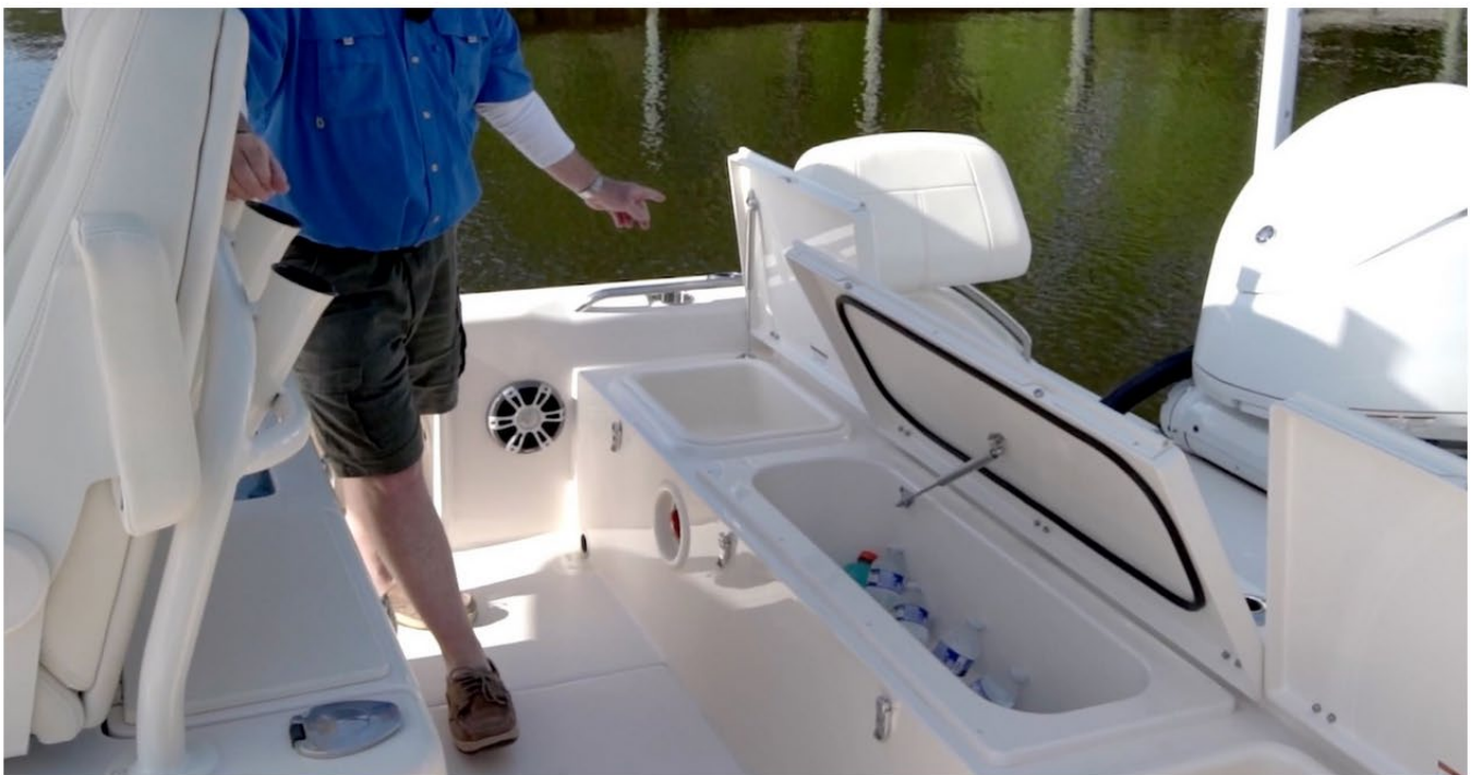
Under the transom bench seating is storage, including an 18-gal (68.13L) insulated cooler. By removing the side bins, we gain access to the bilge area.
