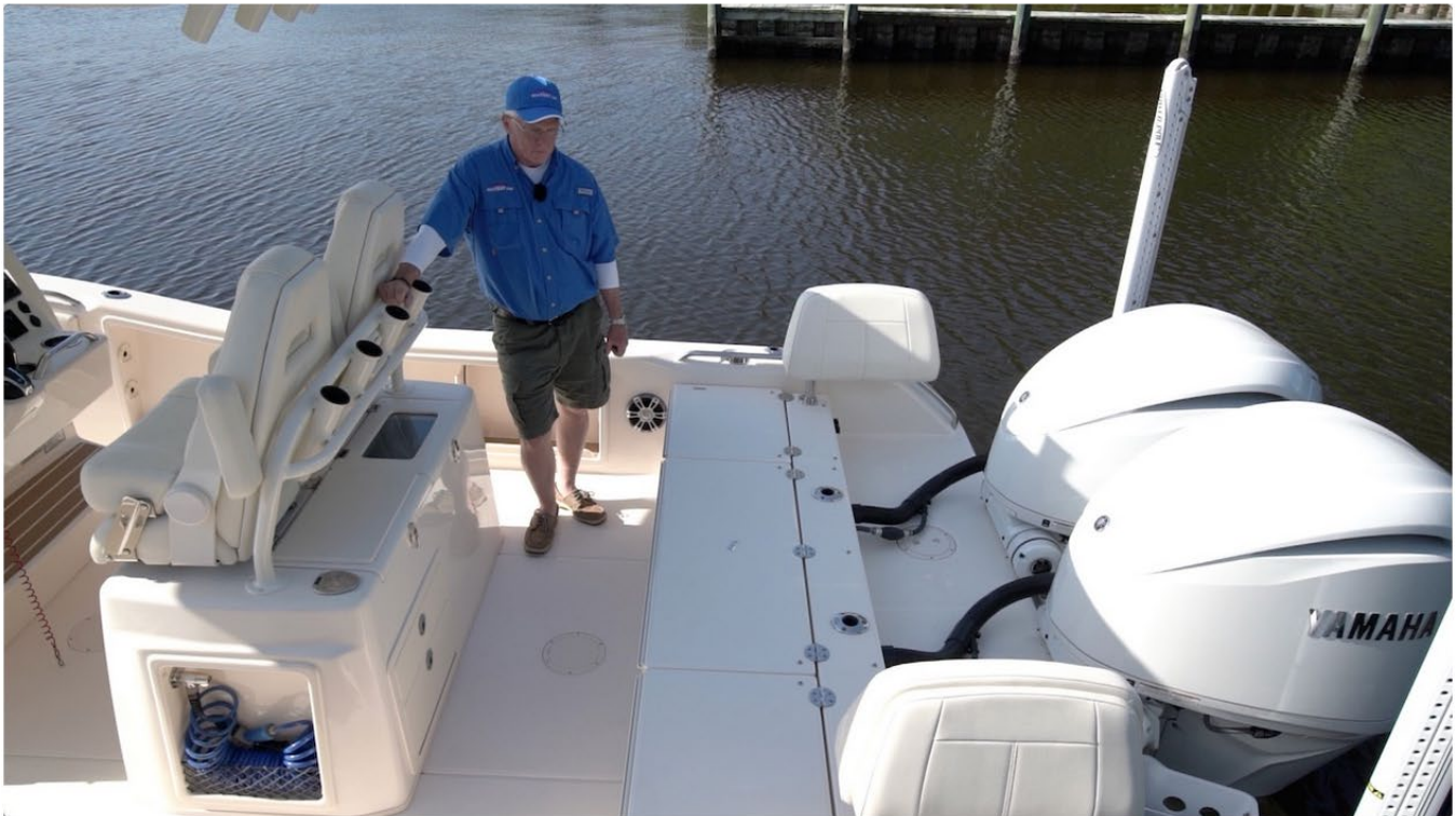
The aft casting deck actually has two levels thanks to the absence of an engine well. Notice how the side seatbacks are swung outwards to make leaning bolsters.
