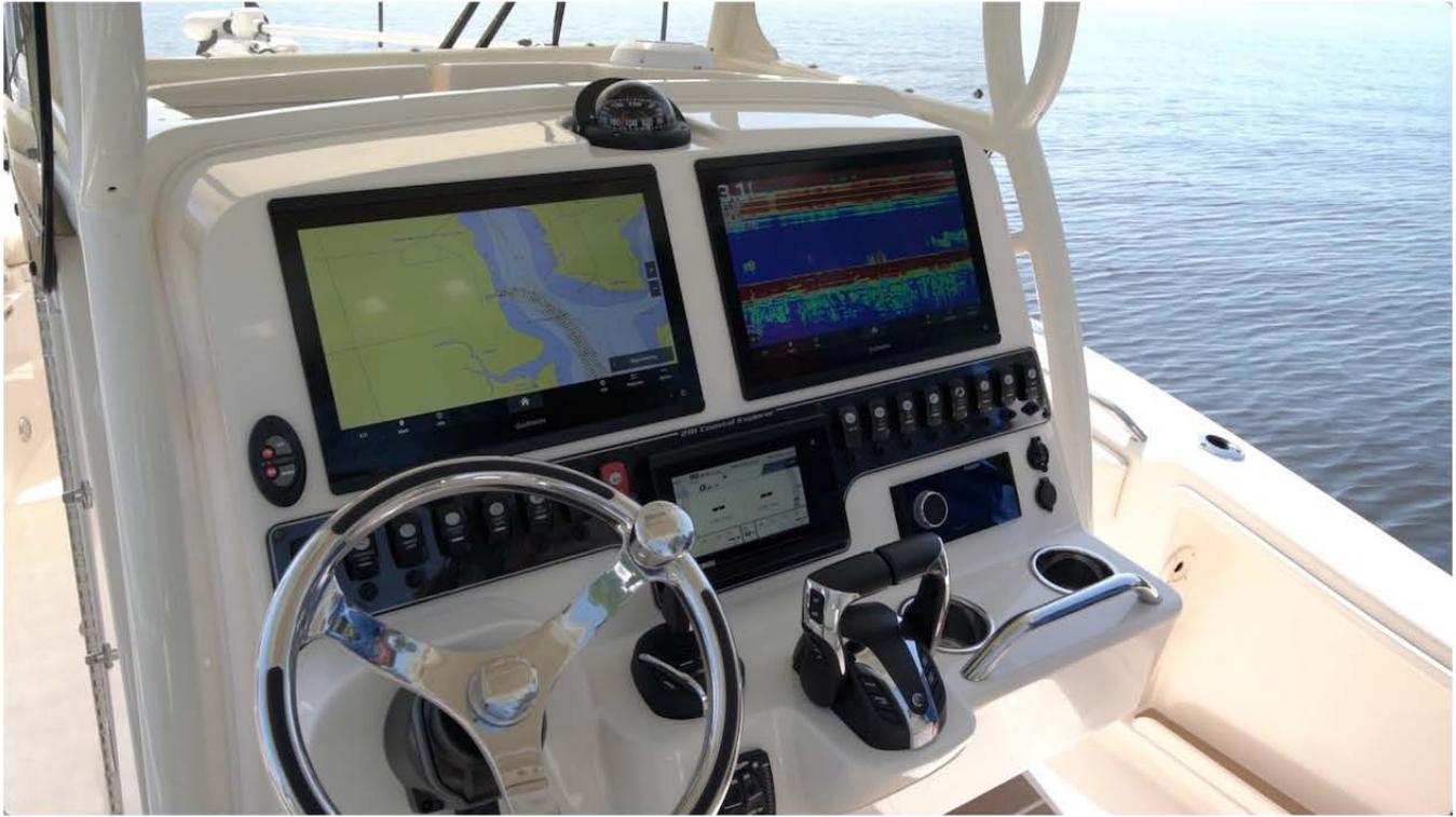
The helm has room for dual 16" (40.64 cm) displays and notice how the switches are below, not above the displays.
