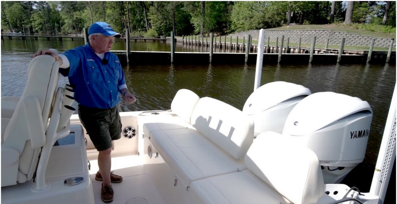
The aft bench seat can seat five across. Notice the center backrest which is supported by a pair of pedestals that insert into rod holders.
