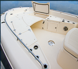
The starboard compartment below the bow casting deck holds four large tackle boxes.
