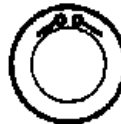
NIGHT VISION DOME LIGHT LIGHT MANF., GUEST REPLACEMENT BULB # GUEST 9-13690 OR GE 912
