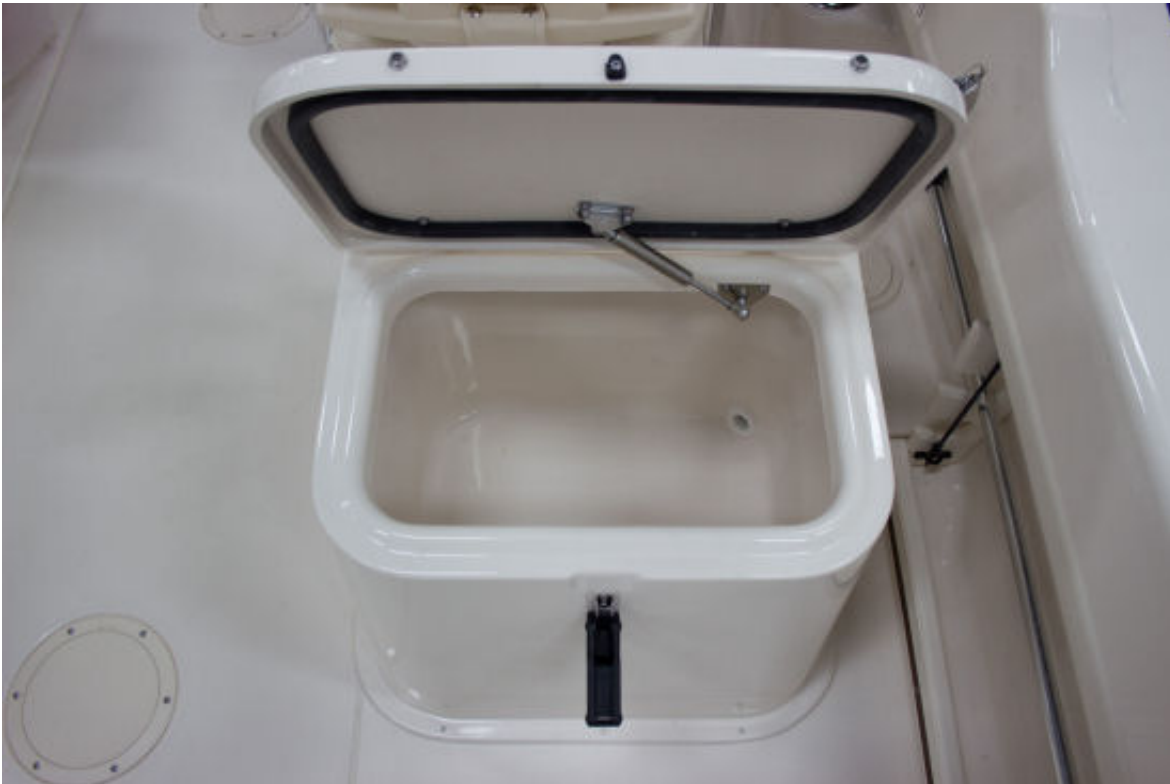
Anglers will particularly like the optional 13-gallon (50 L) starboard insulated raw water livewell with cushion.
