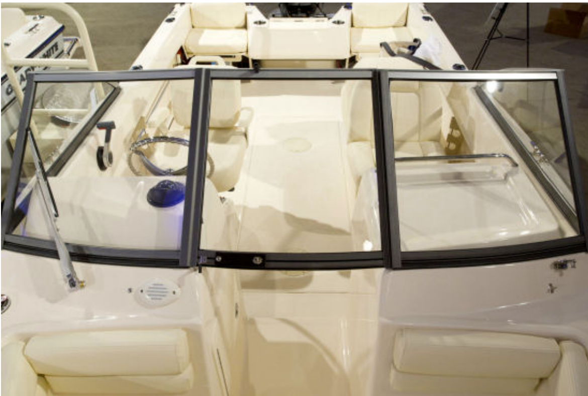
While she is one of the smallest Grady-Whites built she has a remarkable amount of cockpit room because she is outboard-powered. Note the rod holders and rod racks under the gunwales.
