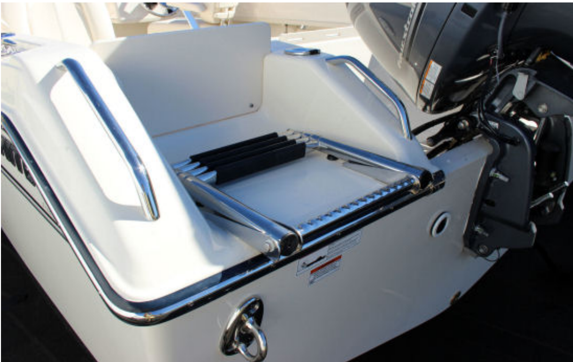
The integrated outboard mounting system with the standard swim platform and ladder. We like the two hand-holds left and right of the ladder.
