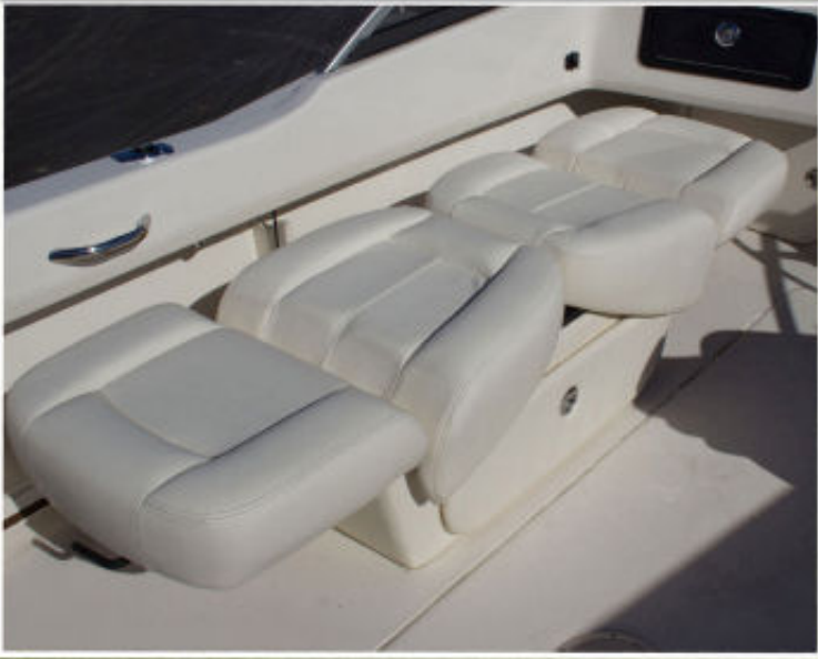
The Freedom 192's optional port sleeper seat is horizontally adjustable with a fore or aft facing backrest and a storage drawer.
